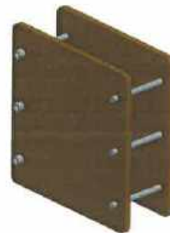
Fig. 2 Diagram of the clamp covered with insulation film 图 2 电池夹具包绝缘膜图
